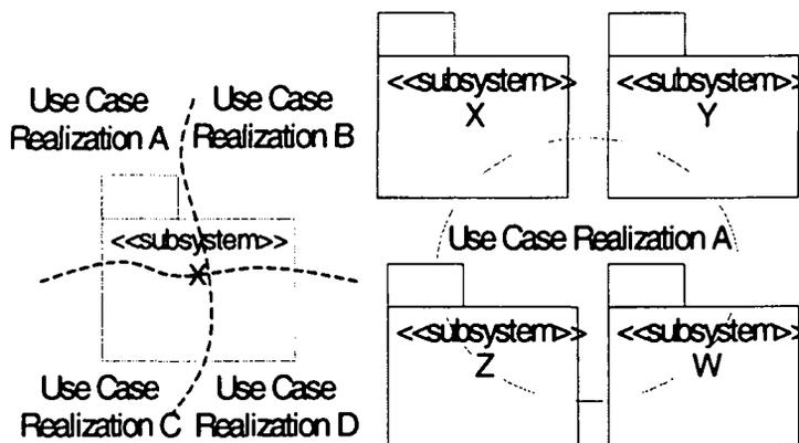
Figure 16. Relationships between physical subsystems and use case realizations
