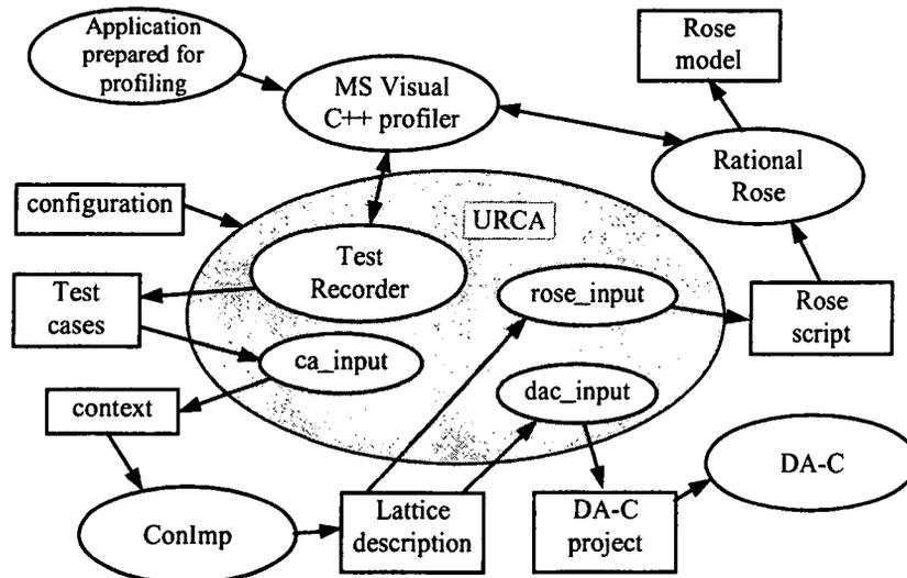
Figure 1. Structure of the prototype system
