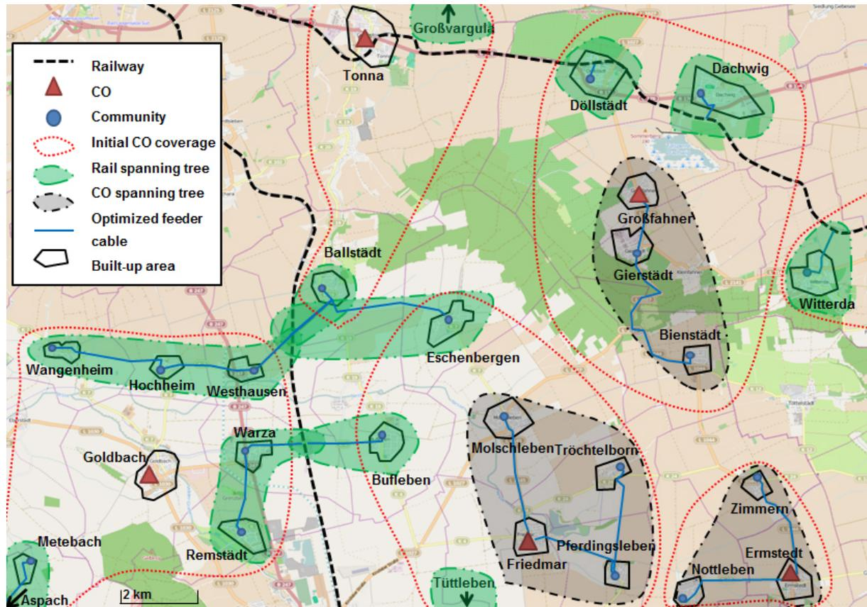
*Fig. 3 Optimized rural feeder cable topology in Thuringia (Germany)*
