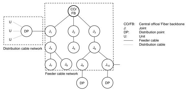
Fig. 1 Typical access network topology in rural areas (adapted from Vidmar et al., 2010)
