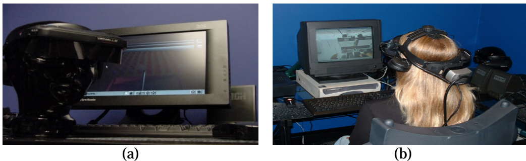
Figure 1. Depicts (a) A Traditional Virtual Reality Environment system and (b) A participant wearing a head-mounted display and head-tracking device immersed in the Traditional Virtual Reality Environment.
