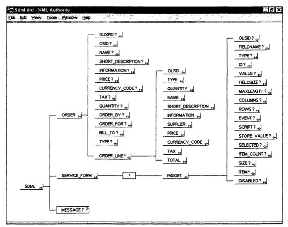
Figure 7: Document Type Definition of an SDML
