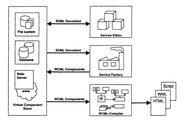
Figure 9: System architecture
